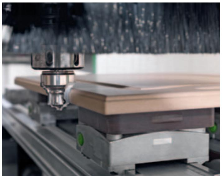
Machining of core panel and element door.
