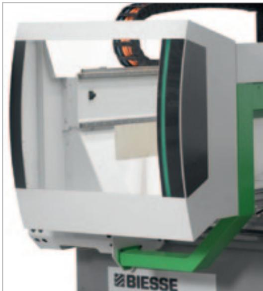
The full protection of the operating units allows maximum visibility to work in total safety.
