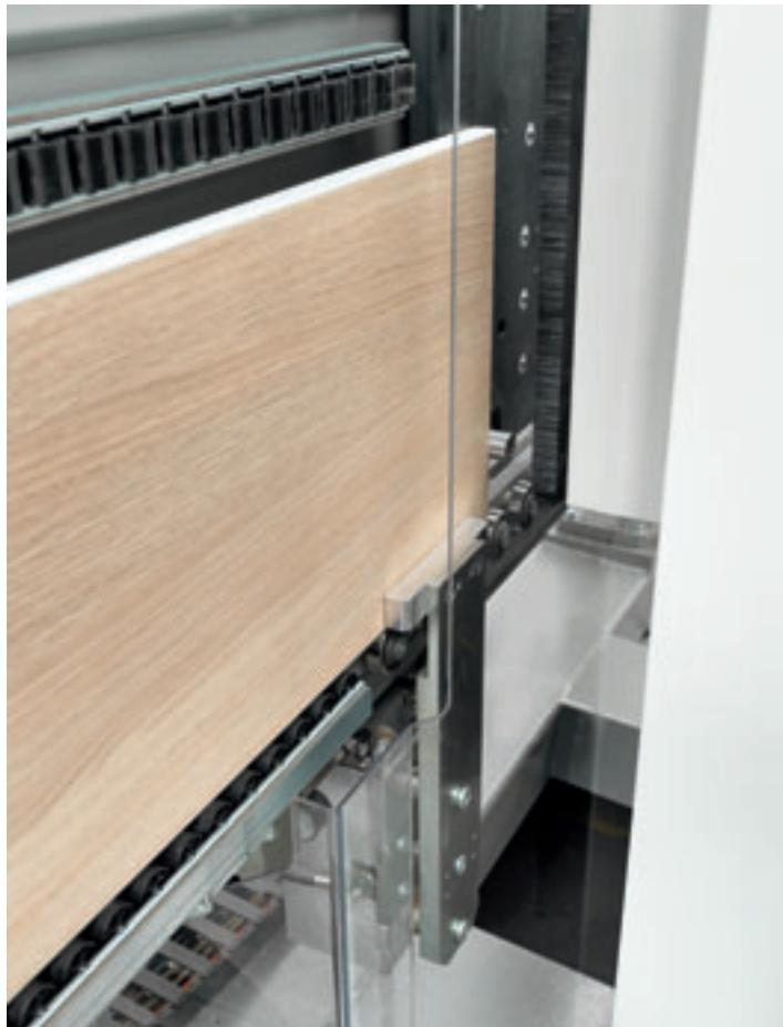
**Skipper V31** is the ideal solution for "just in time" production: set-up time = zero thanks to the panel handling by a fully automatic gripper.
