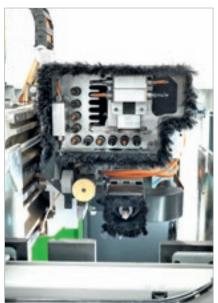
The BH17 operating section, configured with 10 independent vertical spindles + 6 horizontal spindles, along with 1 blade unit (diameter 120 mm - spindle optional), completes all of the machining operations on each of the 5 sides of the panel in a single step.
