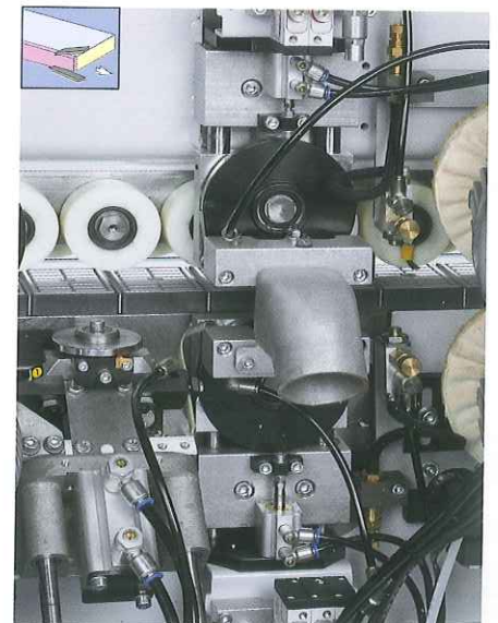
Glue joint scraping unit (optional) For the perfect finish and for edge scraping up to 0,3mm.
