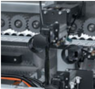
Profile scraping unit
