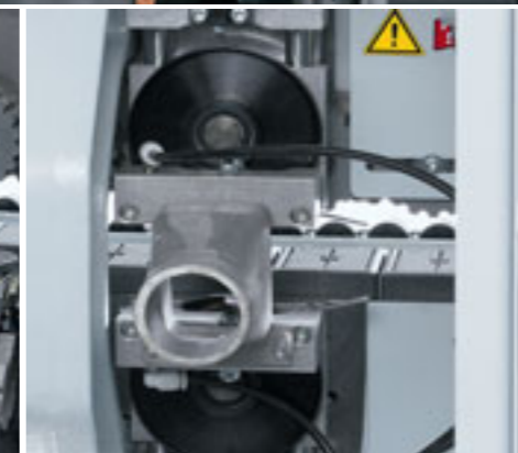
Glue joint scraping unit (optional) For the perfect finish.
