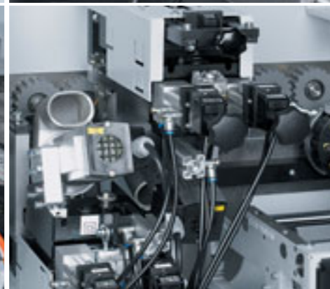
Trimming unit with pneumatic 3-point adjustment (optional) For even more effective production and much shorter changeover time.
