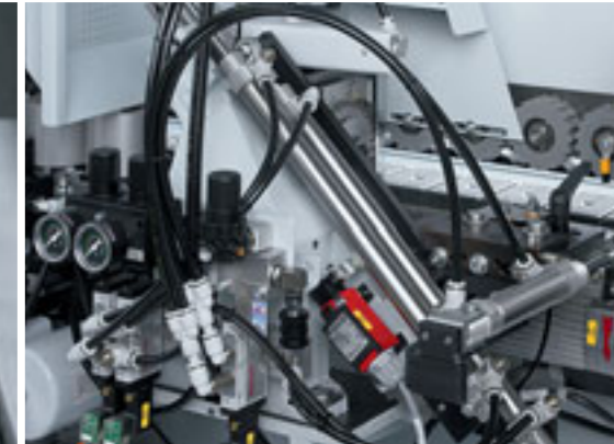
End-trim unit Precise end-cut through a strong end-trimming unit, equipped with THK guides. Chamfer/straight adjustment by easily tilting the unit. (Pneumatic adjustment optional)
