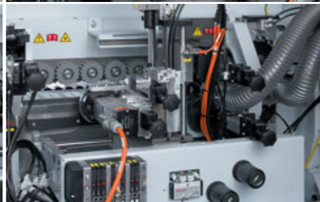
Corner rounding unit FF 10 Optimum corner rounding without adjustment or set-up, resulting from the coupled diamond tool and tracer roller. Workpiece thickness up to 40 mm (optional 60 mm - Ambition 1230 FC).
