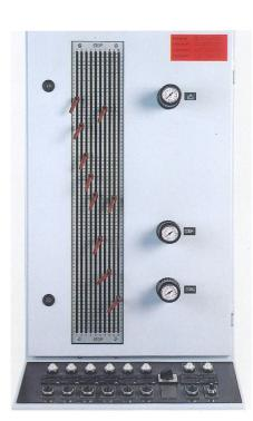
PF machines can be reset within an extremely short period. Our models PF10/42 and PF20/31 have a machine control with mechanically adjustable stop positions and time relay, which controls the cycle itself. Each profile can be written down on a data sheet and therefore each cycle can be repeated at any time. Optionally both machine types can also be equipped with an electronic control.
