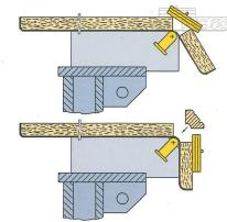
edge and protruding surface material of the panel by means of a spray gun. After clamping the panel into the machine, the surface material is formed around the profiled edge and pressed onto the panel by means of a flat, electrically heated and flexible pressure bar. The pressure bar is heating up the surface material up to forming temperature by means of contact
