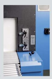
The set temperature is maintained accurately by a closed loop, digital temperature controller; the heating can be set at a temperature of up to a maximum of 250 °C.
