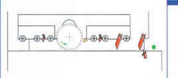
TOP ROLLERS GROUP raised automatically, with 6 independent hold-down rolls and a long wooden shoe placed between the blades. The splinterproof system consists of steel fingers distributed on 4 top rows (two of which acting as splinterproof and the other two as anti-kickback) and one bottom row.
