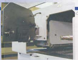
Phe ball-bearing support offers further stability to the spindle which is already overdimensioned.
