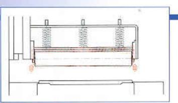
The rollers are guided at the side and they exert pressure over the entire width of the plank through three springs. This application also guarantees good holding of the planks which become curved after drying.
