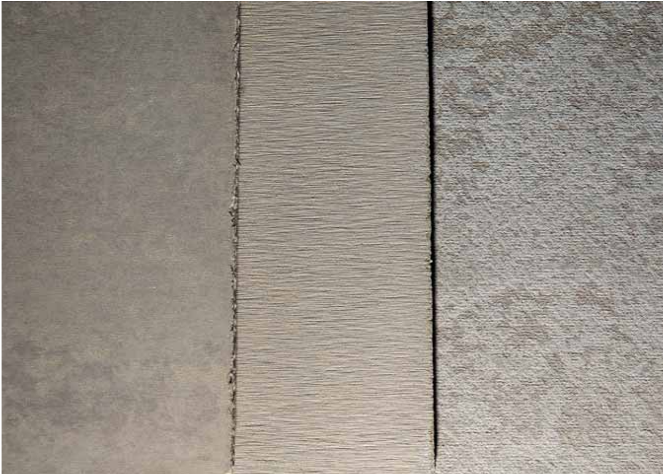
The high power motors (up to 90 kW) and the wide choice of machining units allow users to achieve various finishing effects even at fast production speeds such as 60 m/min
