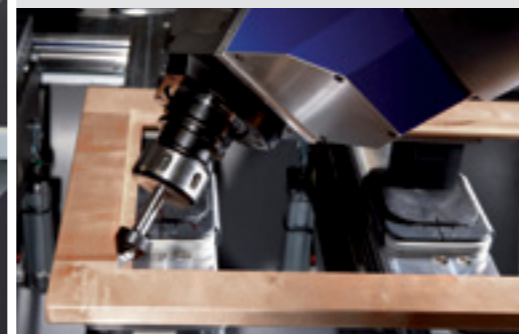
Square corner routing for a glass rebate
