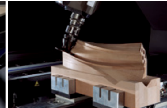
Routing of a stair hand rail
