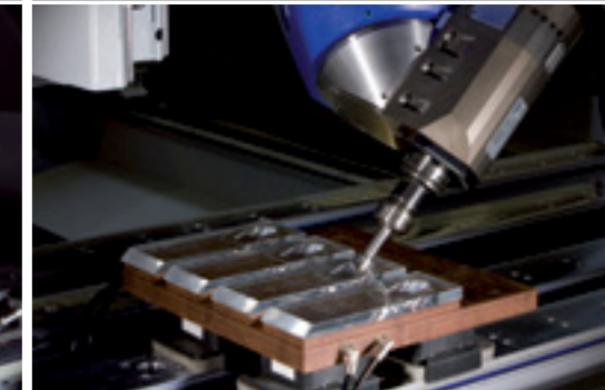
High-gloss trimming of acrylic parts
