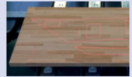
Laser projection of the clamps and the workpiece contour for optimum utilization and simple positioning of raw parts which cannot be aligned at the stops.
