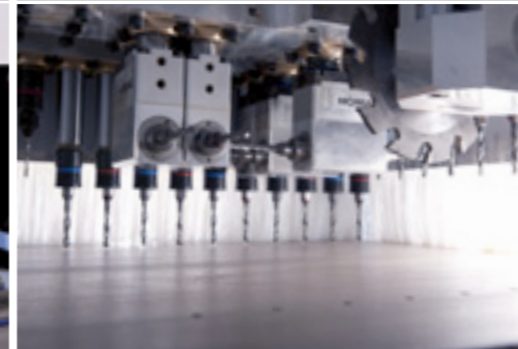
High-speed drilling technology with grooving saw
