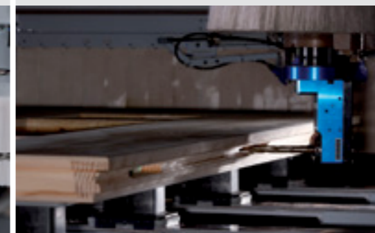
Lock case trimming on front doors
