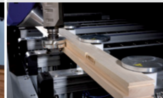
Profiling of frame components
