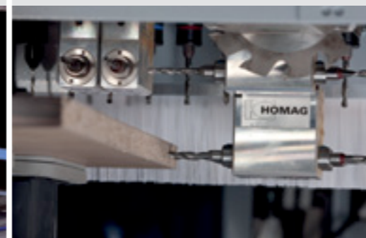
Horizontal boreholes for carcass connections
