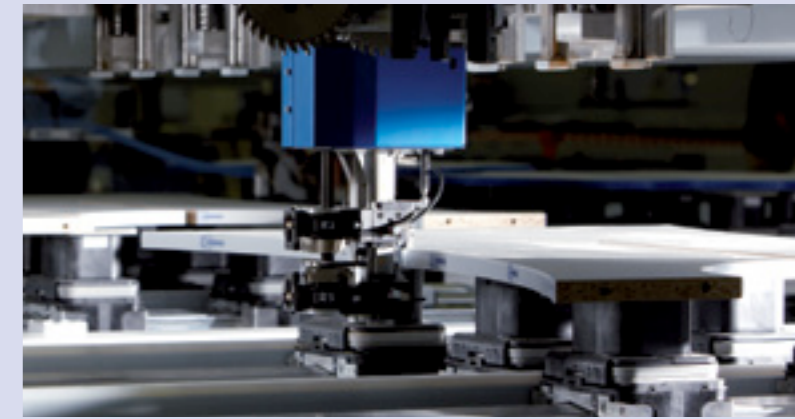
Perfect edge finish due to traced combination flush trimming / scraping unit – efficient processing without tool change.
