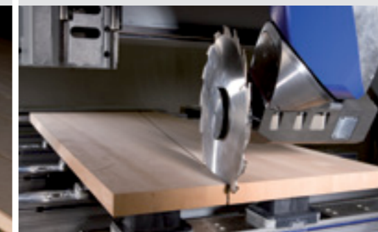
Dividing cuts up to 110 mm in height
