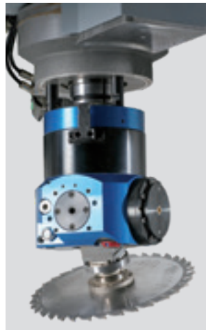
Extension to FLEX5 consisting of FLEX5 interface and FLEX5 unit
