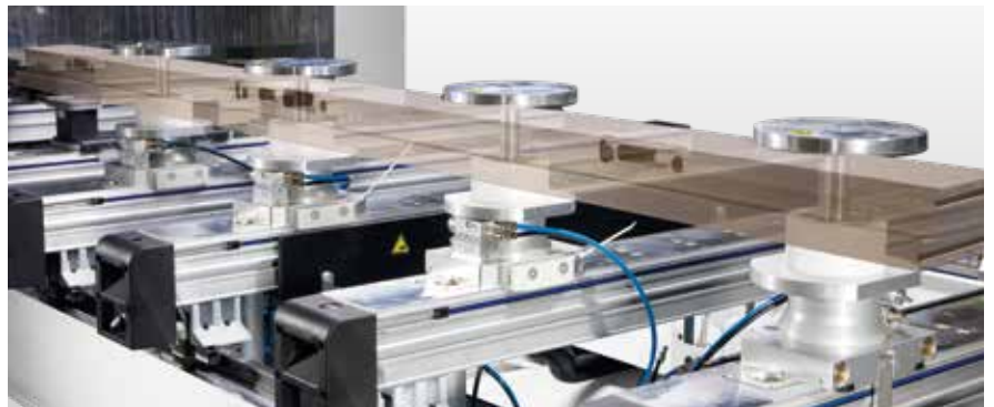
powerClamp manual clamping device for straight and curved parts. Ideal for all curved, narrow and frame parts.
