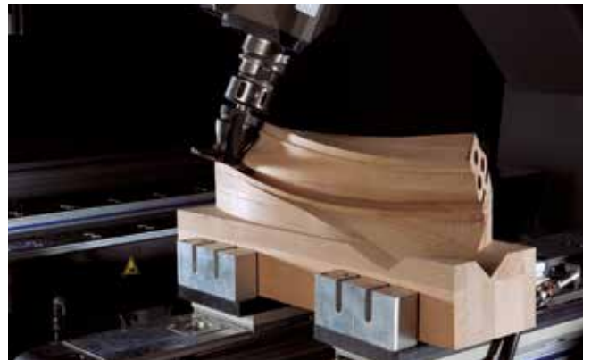
Routing a staircase handrail
