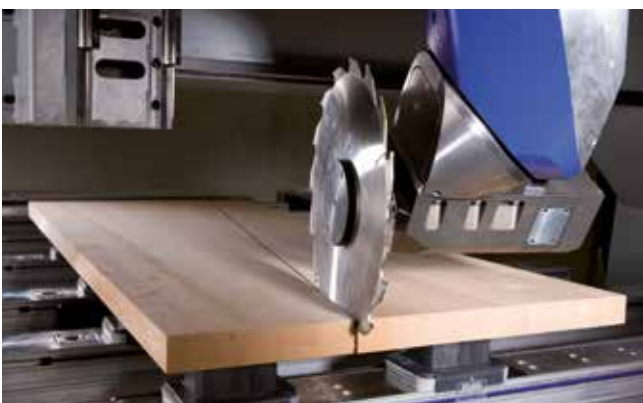
Separating cuts up to 110 mm in height
