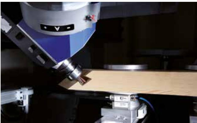
Routing a burr connection for jamb/rail designs
