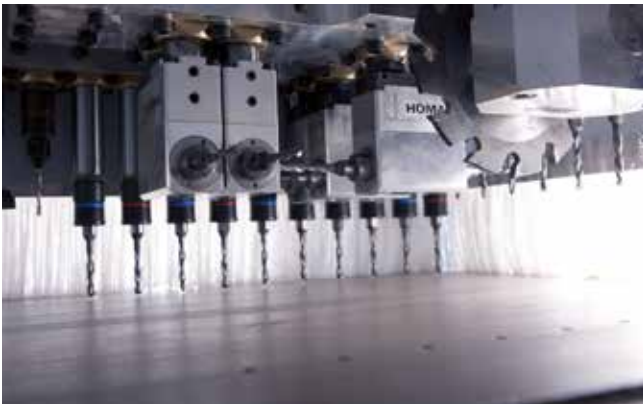
High-speed drilling technology with groove saw
