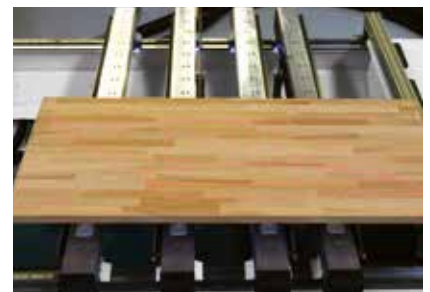
Laser projection of the clamping equipment and the workpiece contour for optimal utilization and simple positioning of unprocessed parts that cannot be aligned on the stops.
