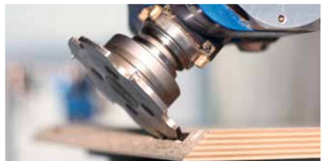
Cutting recesses for connecting fittings
