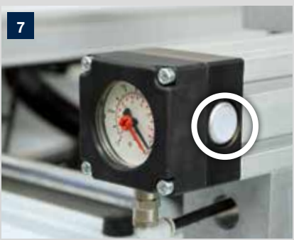
Button for program start – each one at the left and right hand stop profile act as program start for the processing.
