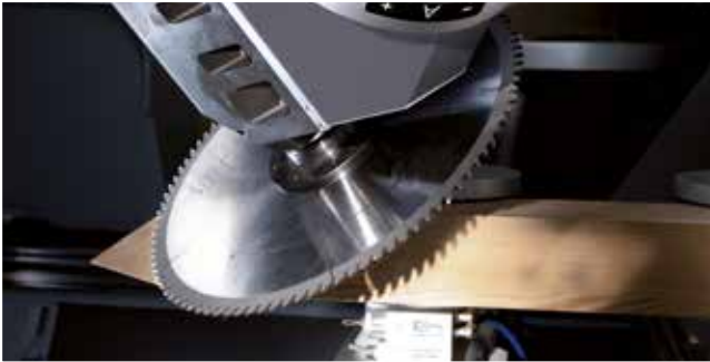
Mitre cut with high cutting depth for frames
