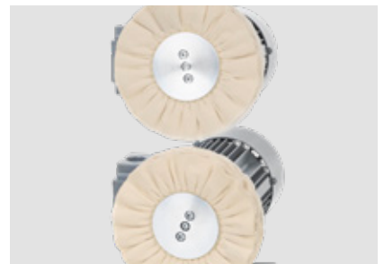
Buffing unit To polish edges and maintain their natural color.
