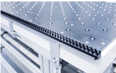
Braking brushes for air cushion table
