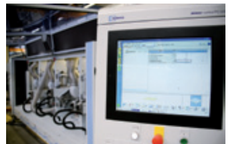
Easy-to-operate powerControl system in accordance with IEC 61131, with facility for remote service and diagnosis
