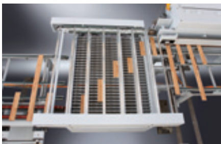
Shifting station from fixed stop side right to fixed stop side left
