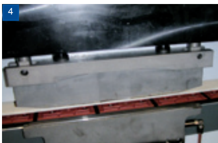
Pressure and support pad for laminate flooring to protect the chain and ensure precision processing
