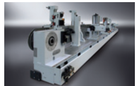
Support frame for flexible equipment of units on the machine bed
