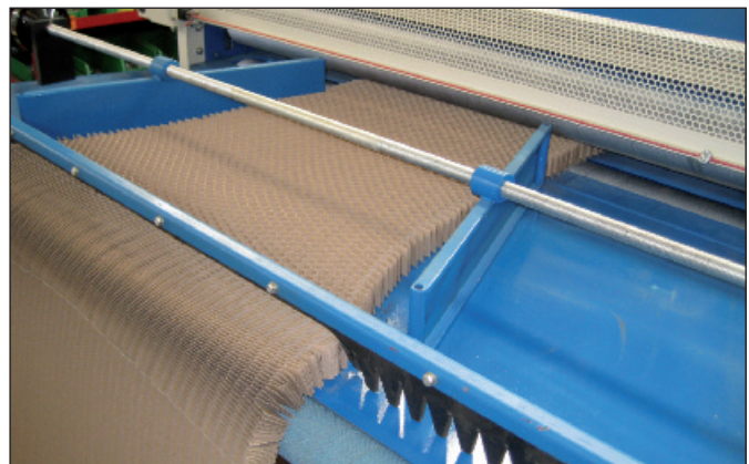
Expanding channel for paper hexagonal honeycombs
