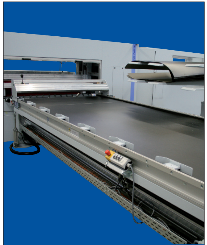
Positioning belt, double-sided glue application
