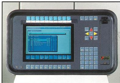
The PC series offers the user the possibility to fully automate unit positioning so as to set the units automatically to various edging materials (no manual adjustments, readjustments), as an optional extra.
