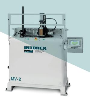
A specially designed boring and inserting machine to fit screws and bushes into sofa legs, feet etc. The standard machine is equipped with a bottom boring unit, a screw inserting and manual feeding unit (screws M8x70).
