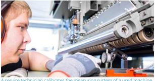
A service technician calibrates the measuring system of a used machine.
