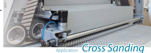
For certain applications, a cross sanding unit proves to be the perfect choice. For example, an unparalleled finish can be achieved on cross-veneered or high-gloss lacquered parts, especially in combination with our patented oblique sanding technology. For this purpose we offer a selection of different cross belt units, alternatively integrated in the machine body or at the machine exit.
