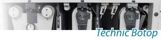
With our *Technic Botop* series wide belt sanding machines, the top and bottom sides of workpieces can be sanded in just one pass. This saves time and effort, which would be required to perform several sanding operations. These systems are very popular with panel production, veneer processors and stair construction companies, for example.
