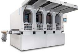
KUNDIG offers a wide range of solutions for the texturing of surfaces. In most cases, brushes are the means of choice. These are available as an additional unit in wide belt sanding machines, either integrated in the machine body or mounted at the machine outlet. Dedicated brushing machines are also part of our product range.
