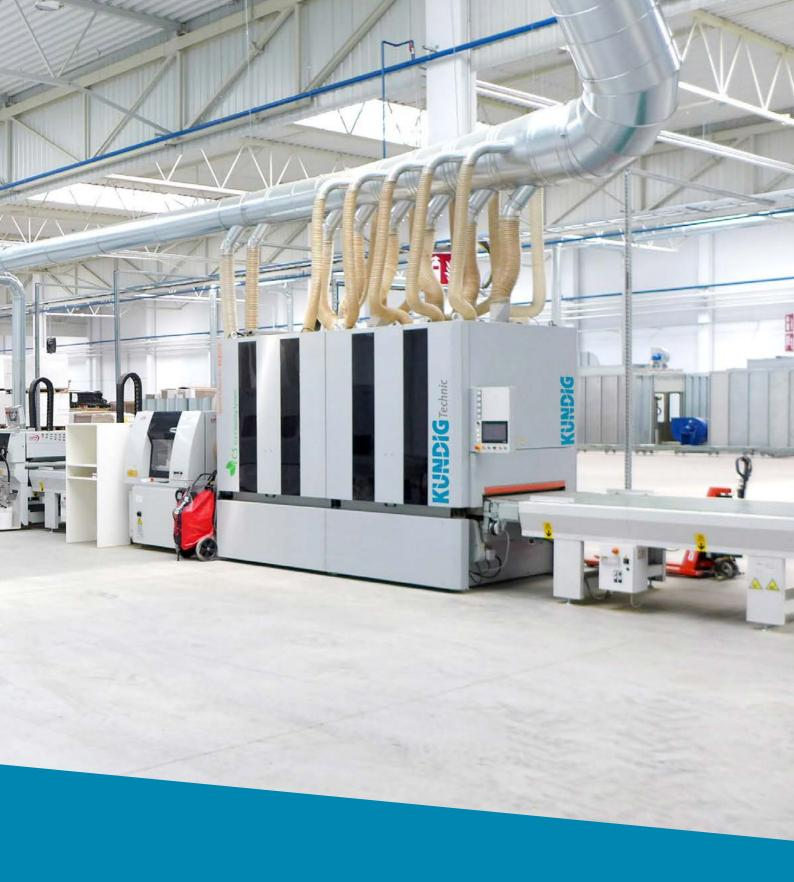
Sanding machines of our *Technic* series are available for all sanding applications and materials imaginable. Whether high-precision sanding with hundredth millimeter tolerances, texturing with an unprecedented repeatability, sanding of abrasive materials or shape sanding with a CNC sanding unit. Our experience covers many industrial sectors and materials. The potential for individualization is vast. Complete custom-made products and special projects are also possible.
