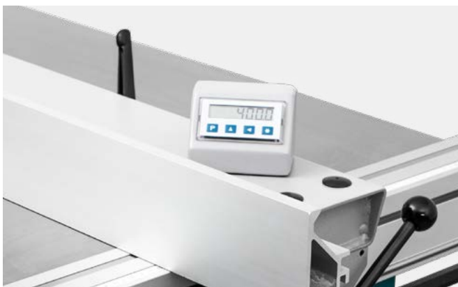
Electronic indication of the cutting width | T60A12
