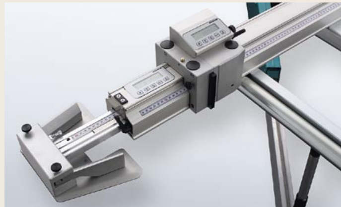
T6042 Digital cross-cut fence with 2-point alignment
