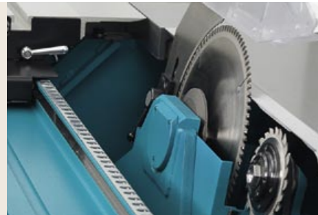
Quick blade replacement with V-Lock
