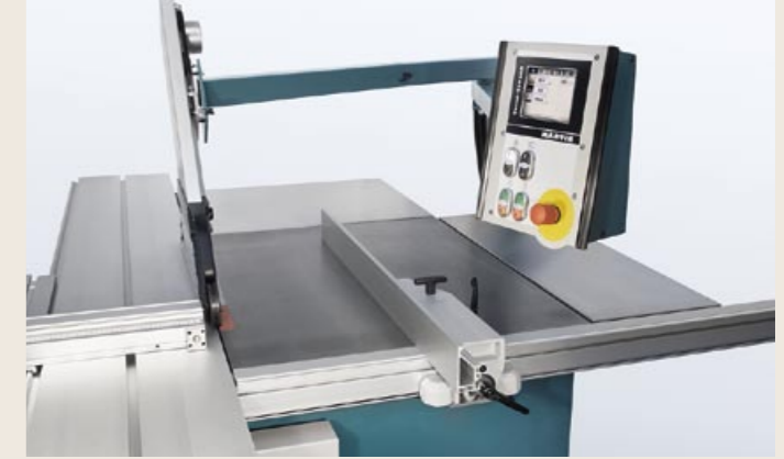
T6090 Motorized positioning of the rip fence
