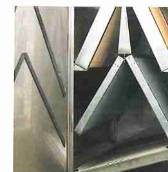
The high efficiency filters separate the varnish particles from the suction air, to be recovered.
