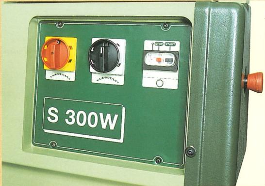
All CE machines are fitted with a lockable main machine switch, magnetothermic overloads, start/stop device and emergency stop pushbuttons in the operator zone.
