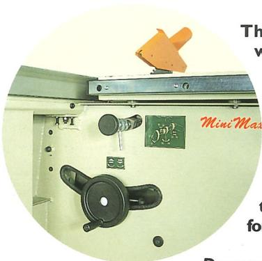
The scoring blade, which can be adjusted from outside the machine guarantees rapid, easy setting-up in complete safety and without leaving any play. No tools are required for this adjustment.
