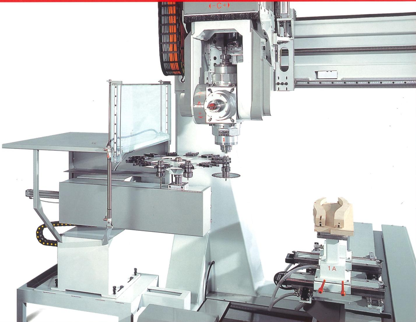
SPIN is the open beam structure workcenter particularly meeting the high standards of manufacturing chair and table components as well as solid wood elements in general. It has been designed for precise 5 axes interpolated machining operations: boring, mortising, tenoning, shaping with unrestricted three-dimensional manoeuverability. The dynamic conception of SPIN offers a higher degree of flexibility ideally suited to machining also plastic articles.
