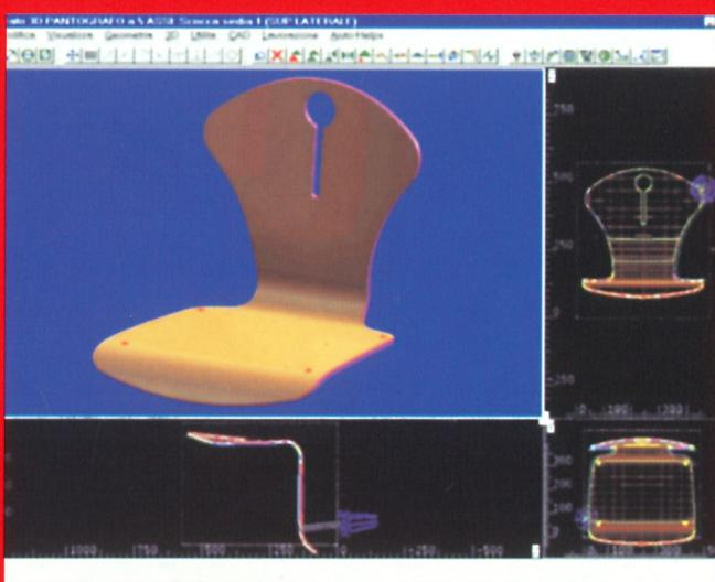
More complex milling operations are to be programmed by means of CAD/CAM operative station, that is usually interfaced with a three-dimensional digitiser in order to detect shapes directly from a sample.
