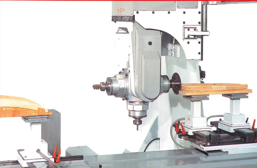
The machine is supplied with two separate tables that work independantly (axes Y1 and Y2) processing the production in pendulum: while the machine is working on one table the component can be changed on the other, eliminating 'idle time'. When necessary the tables can be united in 'gantry' where they move together simultaneously hereby creating a unique work area for larger components.
