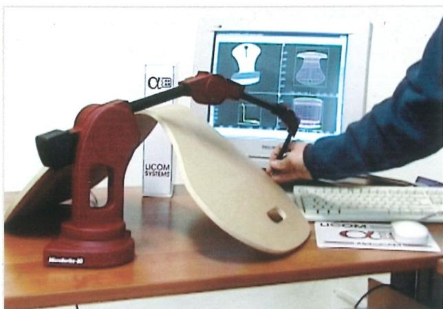
More complex milling operations are to be programmed by means of CAD/CAM operative station, that is usually interfaced with a three-dimensional digitiser in order to detect shapes directly from a sample.
