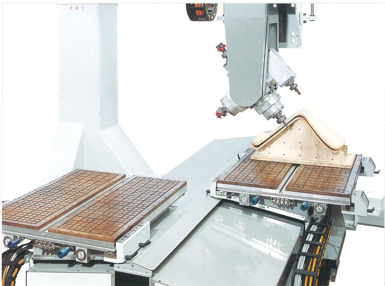
**S**PIN is the open beam structure workcenter particularly meeting the high standards of manufacturing chair and table components as well as solid wood elements in general. It has been designed for precise 5 axes interpolated machining operations: boring, mortising, tenoning, shaping with unrestricted three-dimensional manoeuverability. The dynamic conception of SPIN offers a higher degree of flexibility ideally suited to machining also plastic articles.
