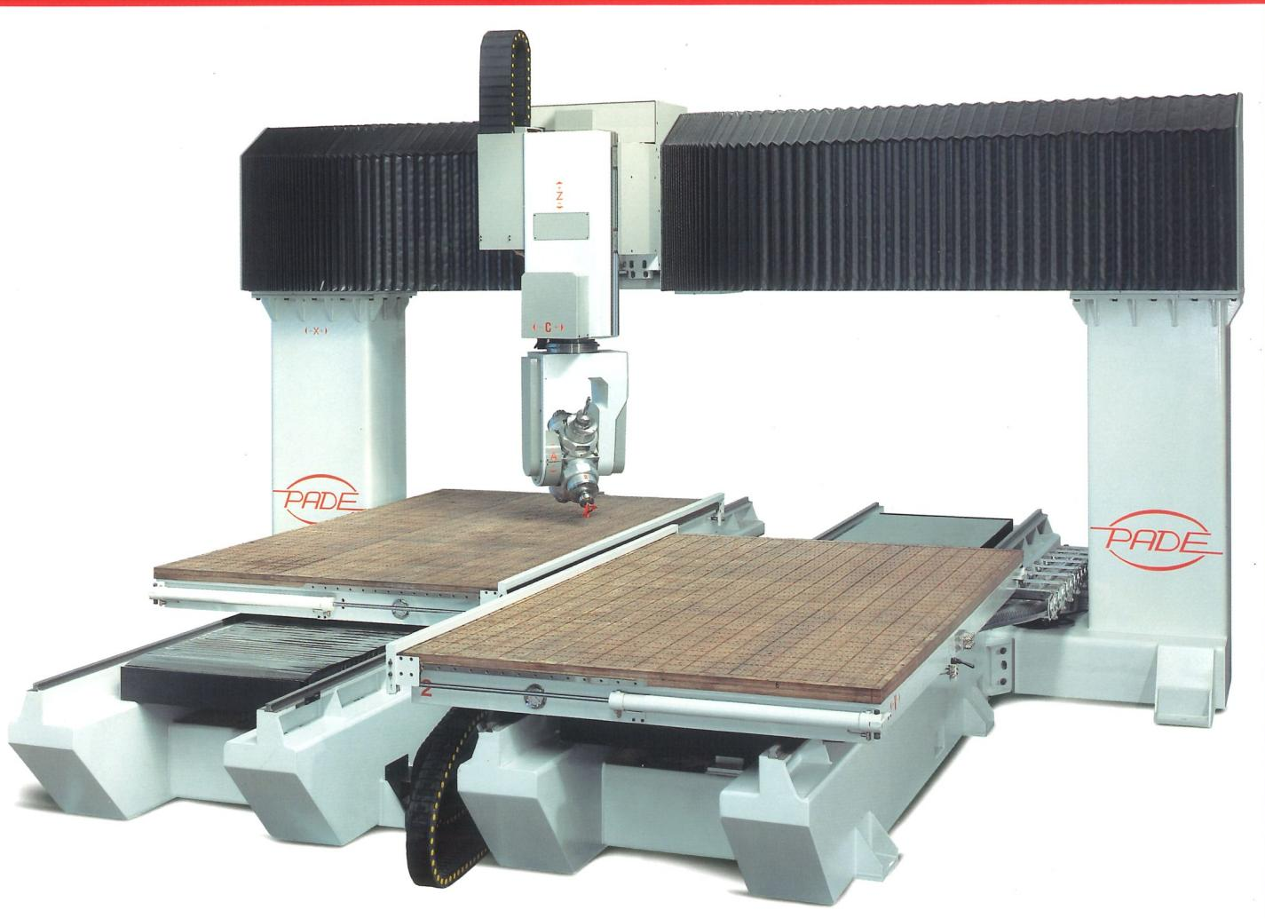
The TOP Working Centre is the ideal solution to process large-sized pieces on 5 axes. The machine comes complete of a single-spindle head with an automatic device for tool changing and a large capacity store to guarantee the working maximum flexibility. In alternative, solution is available that provides a head with a turret system and 4 independent motors, a solution that stands out on the
