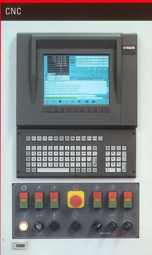
Numeric Control is supplied with all software options to allow the machine to work the most complex pieces simultaneously on 5 axes.
