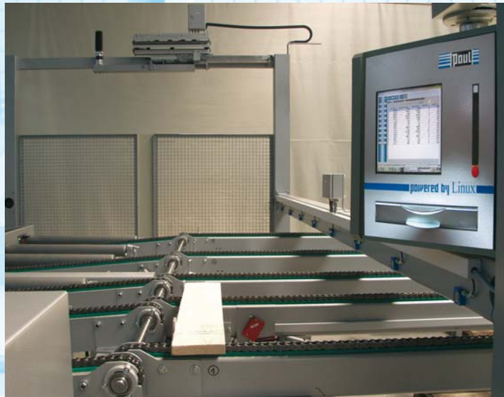
Fig. 8: The laser portal is positioned by means of a servomotor. The lasers can be slightly adjusted, in order to reflect the saw fixing
