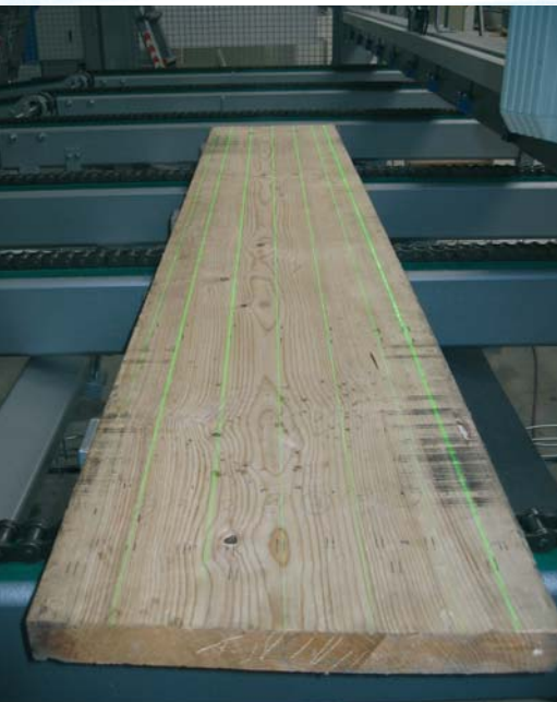
Fig. 3: The laser sensors measure the workpiece
