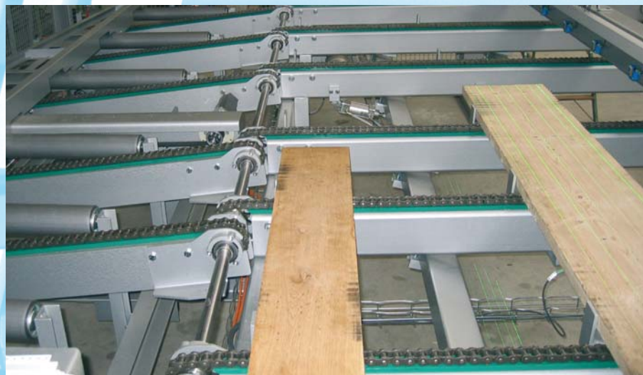
Fig. 10: The stop rail enters into position so that the plank can be fed to the rip saw at right angles and precisely to fit the selected sawing pattern
