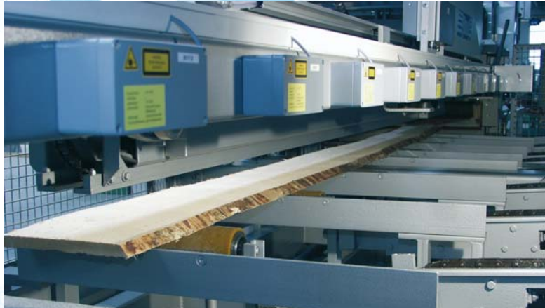
Fig. 2: The sliding carriage positions the workpiece with great accuracy
