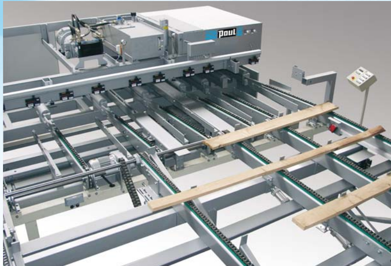
Fig. 6: From 1200F with buffer chain conveyor
