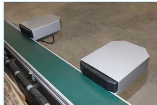
Fig. 12 Fully enclosed ejection stations for high safety
