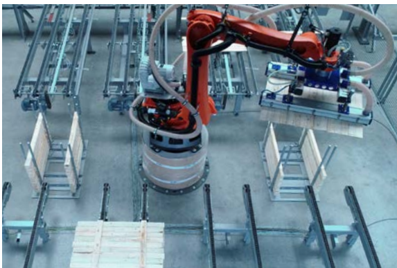
Fig. 6: Articulated arm robot
