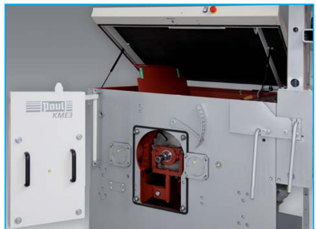
Fig. 13: KME3 with opened machine hood and opened front bearing cover
