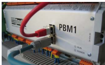
Fig. 5 Connection of the PAUL PBM1 bus module via Ethernet cable
