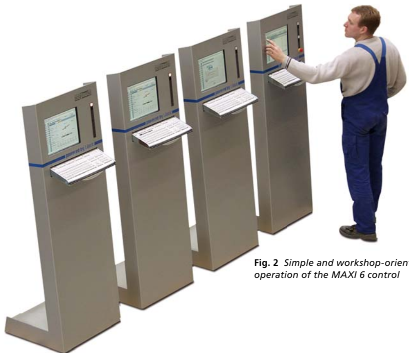
Fig. 1 Operating terminal of MAXI 6 control with touch screen
