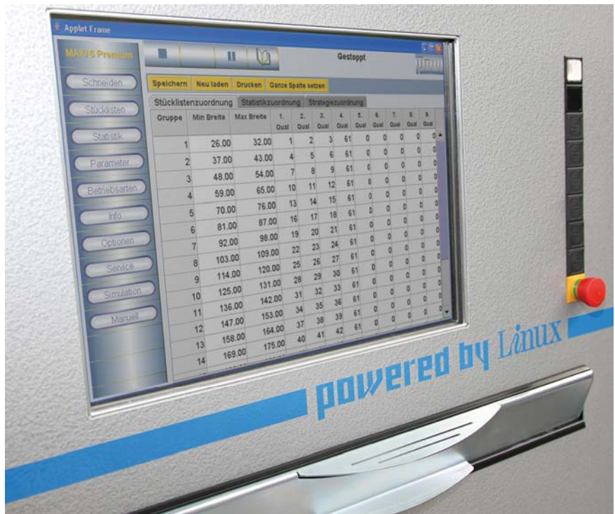
Fig. 1 Operating terminal of MAXI 6 control with touch screen
