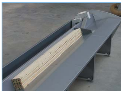
Fig. 4 + 5 Upward tilting standard pusher enables length measurement & crayon mark recognition – also ideal for cutting timber packs
