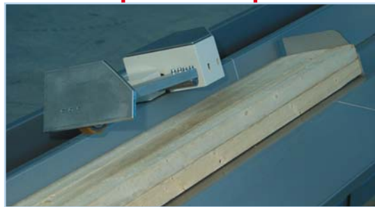
Fig. 16 The output is increased significantly when cutting several pieces packed together
