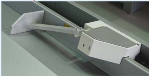
Fig. 15 The upward tilting pusher is fitted with various sensors. It enables length measurement and crayon mark recognition
