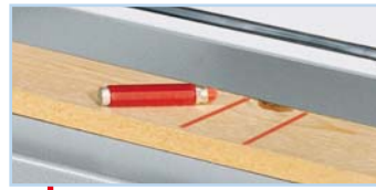
Fig. 11 Marked defects are cut out (option)
