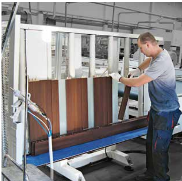
Interior door pre-assembly with action h automatic clamp
