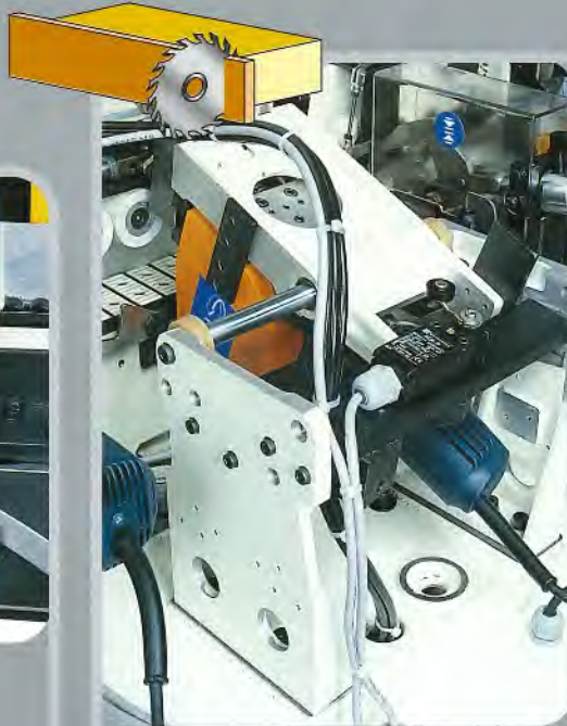
Single-motor end trimming unit with ergonomic and compact design; also has a copier. Available in the electro-tool version (10,000 rpm).
