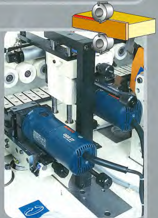
Edge trimming unit. Moves on ground guides with re-circulating ball screw bushes. Available in the electro-tool version (27,000 rpm)
