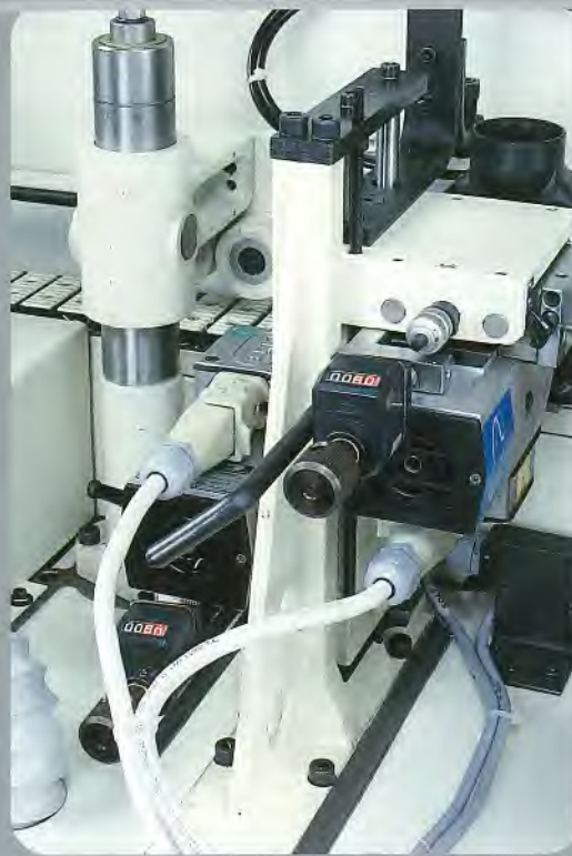
Edge trimming unit. Moves on ground guides with re-circulating ball screw bushes. Available in the high-frequency version (12,000 rpm)
