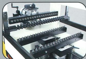
As standard the machine is equipped with a **reference guide** fitted with four pneumatic stops. The stops are selected and controlled from the control panel.
