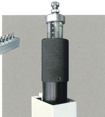
Continuous boring depth adjustment as an alternative to the 6-positions mechanical revolver. (available on request).
