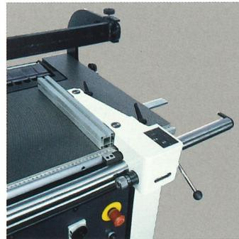
Top positioning precision of reference guides with micrometric travel and Vernier scale adjustment.
