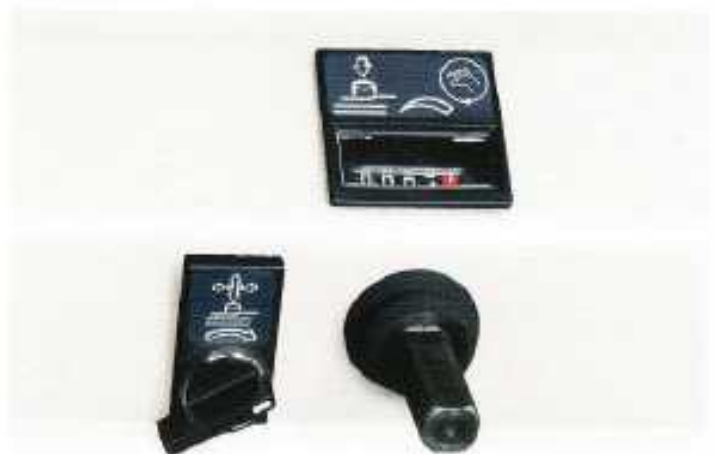
Pneumatic device for spindle locking in working position, positioned on the front of the machine.
