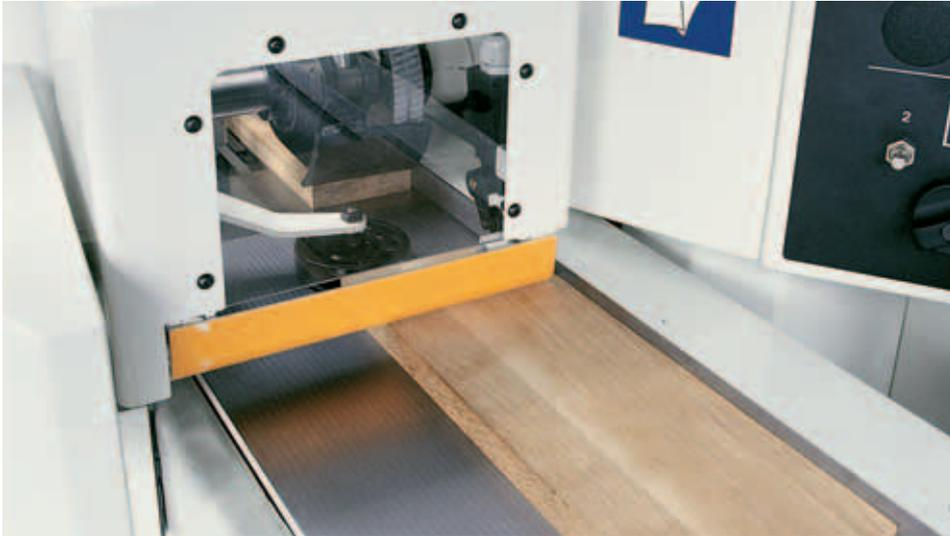
Left vertical spindle with automatic adjustment for machining parts of different widths in sequence.
