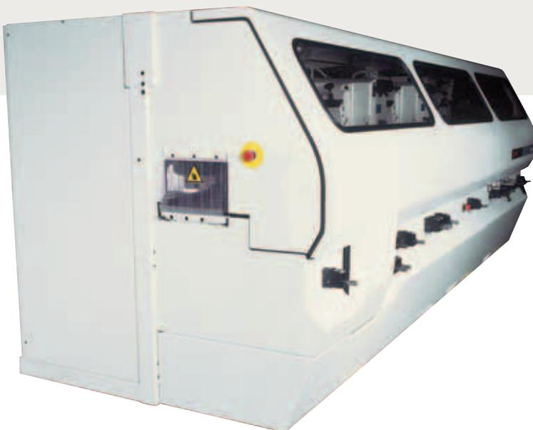
Integral safety enclosure which drastically reduces dust and noise in the surrounding work area and protects the operator from risks.
