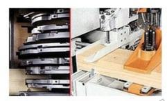
Butting to measure of workpiece length is NC controlled and it is possible to automatically machine 2 components at the same time with automatic rotation. The machine can accept 2 multitool spindles, which can be up to 620 mm. long with outboard bearings and "Jolly" anti-chipping unit
