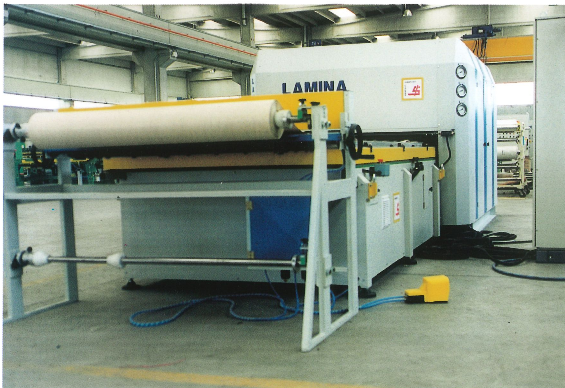
LAMINA, single tray, automatic loading and unloading system. The press can be converted into a double tray system, shuttle right and left.
