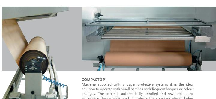
work-piece through-feed and it protects the conveyor placed below and immediately absorbs the overspray. The change over from a job to another is immediate and it does not need cleaning operations, except those related to the spraying circuits.
