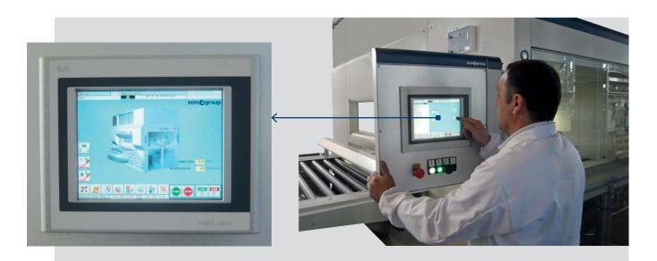
Electronic control via PLC and touch panel; user-friendly software controls the spraying parameters, stores the working recipes, eases diagnostics and programs the ordinary maintenance.
