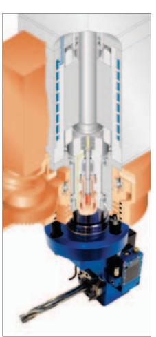
Water-cooled routing spindle
