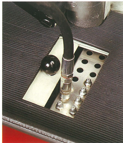
Central location of lubrication points makes preventative lubrication easy. No overlooking of lubrication points, not even those for the axial spindle adjustments.
