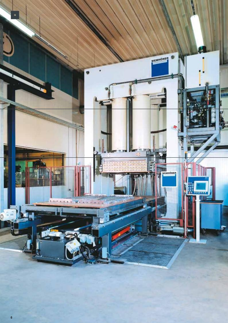
Wemhöner Moulding and Vulcanising Press Lines offer a wide range of applications to manufacturers of composite materials. Rubber-metal, Aramid or GRP composites are only some examples of custom-made products. The specific pressure of these lines are around 650 N/cm² and provide total press capacities of 24,000 kN.
