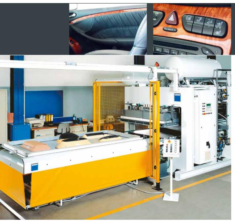
The use of Wemhöner technology in the photovoltaic industry goes well beyond the usual applications in the classic field of surface finishing. In line with today's awareness about environmentally friendly energy, the VARIOPRESS® SolarLam is being used for the production of solar cells. The fragile glass modules are laminated under high vacuum and at an additional pressure of up to 3 bar with maximum accuracy at constant temperature.
