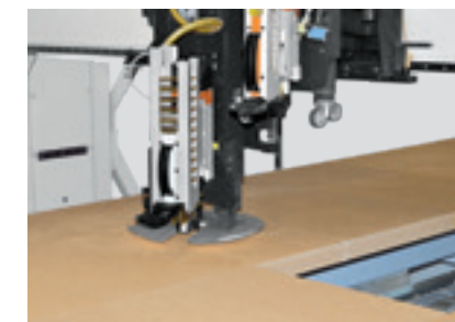
Sliding shoe for attachment devices Fastening to protect the material, especially suitable for soft wood fiber.
