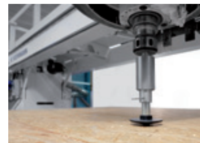
Marking and labeling Marking of panel joints, slat positions, or shuttering boards enables fast and easy positioning.
