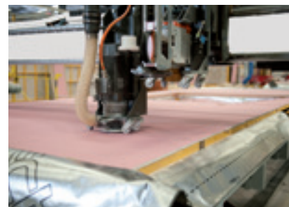
Processing gypsum plasterboard
