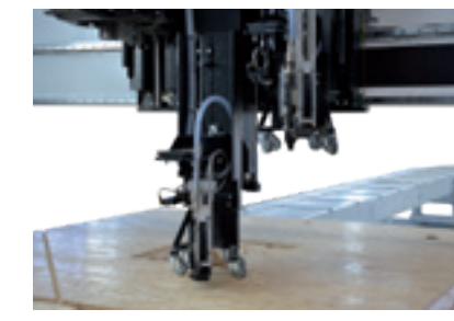
Chuck for a second fastening unit Different fastening units enable the attachment of various types of sheathing material.
