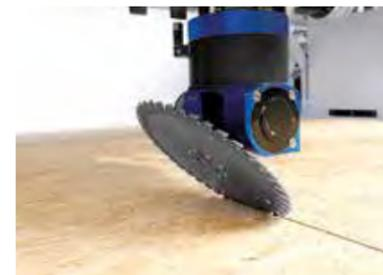
**Flex 5 Sägeaggregat**
