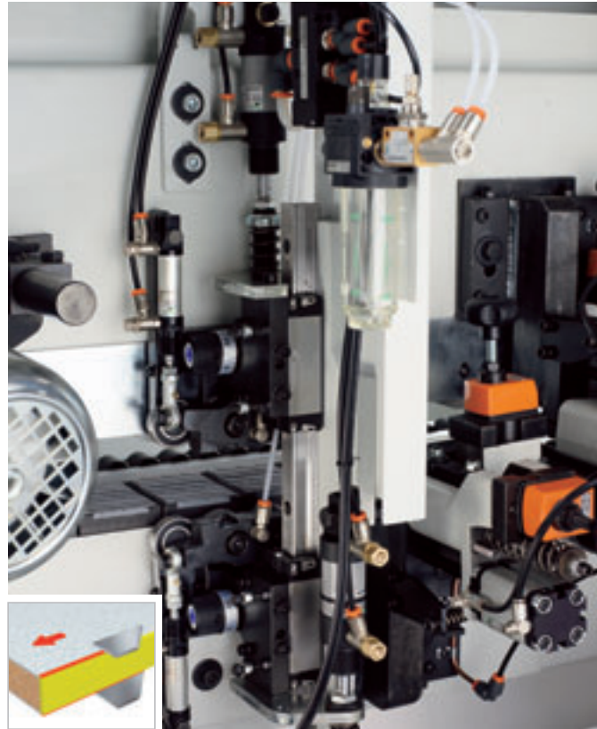
Glue scraper RCC-701. Removes any residual glue using two knives fitted with a timed intervention turning discs copying system.
