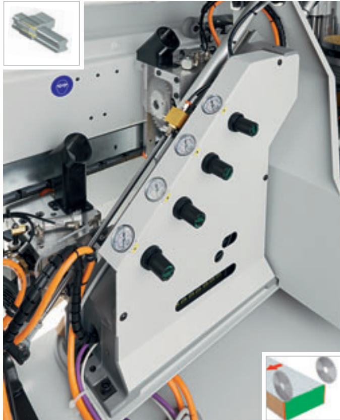
End trimming unit IN-801. The group can be tilted (from 0 to 15 degrees) automatically from the control panel with two independent high frequency motors (0.8 kW each).
