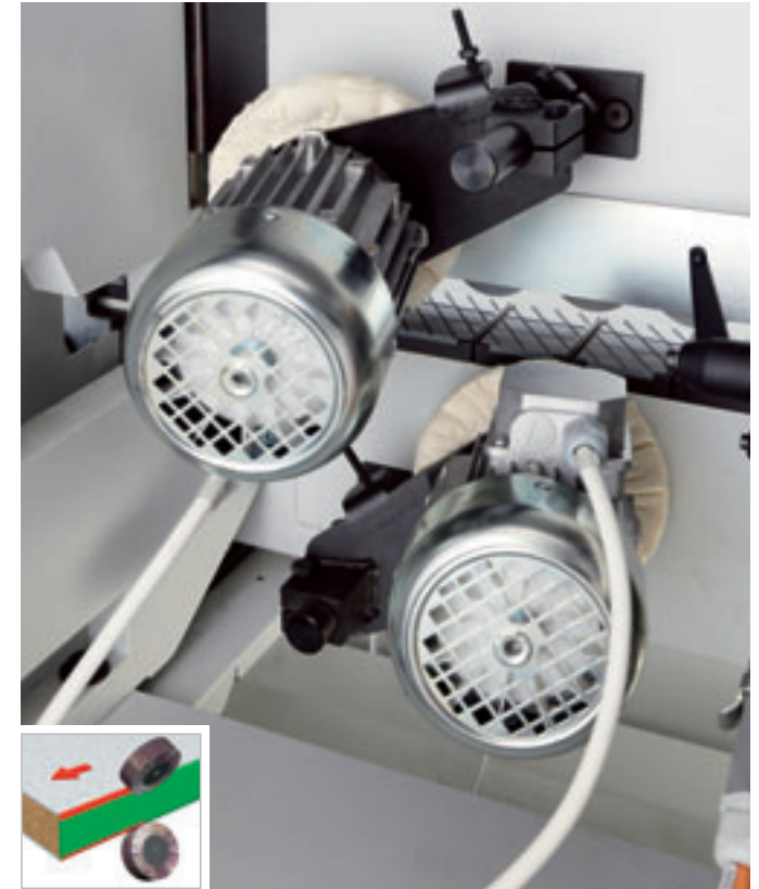
Brush unit SP-501. Tilting brush unit to clean and polish the edge of the panel.
