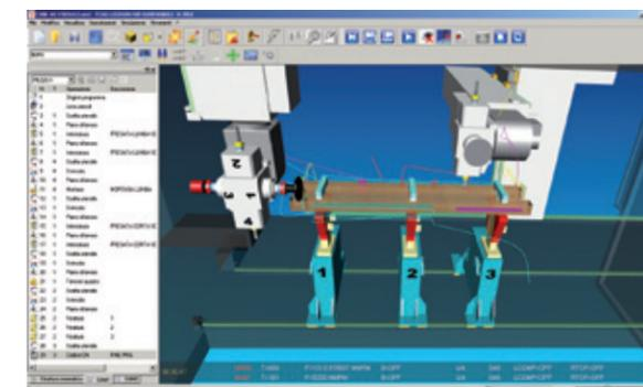
All the features mentioned above can be executed on the machine PC (also during machining) or on another generic PC. It's important to visualize the cycle preview to save time and sample pieces.
